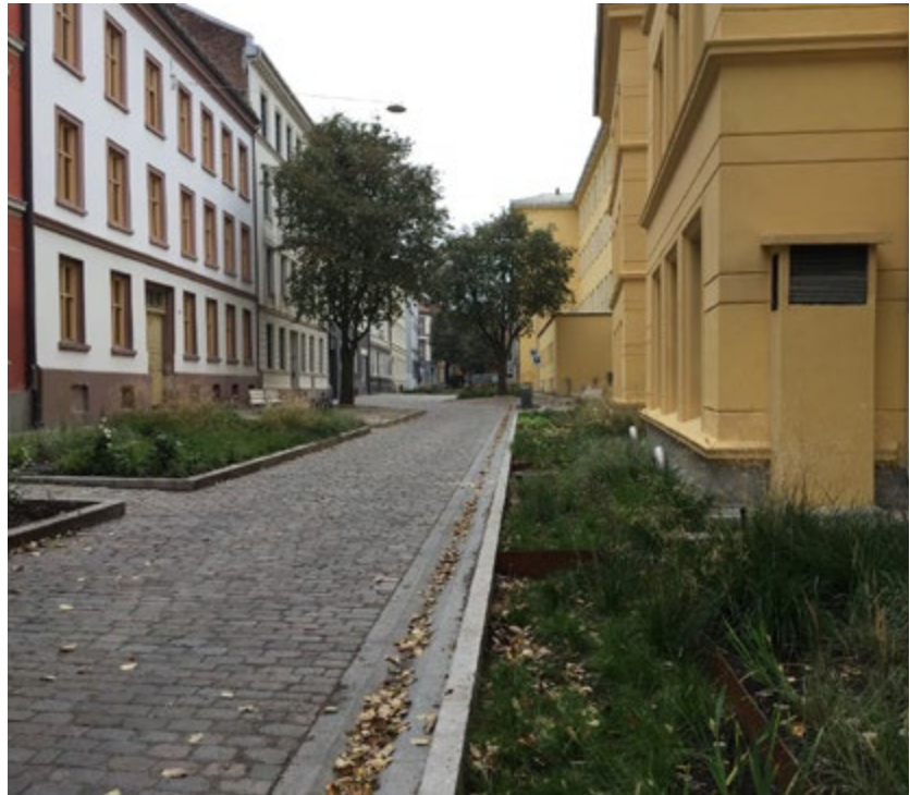
FIGURE 6-5 Example of rain garden in an established street space, Deichmans gate.
