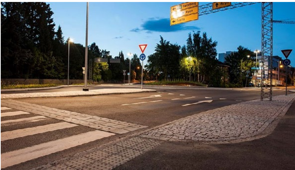
FIGURE 4-2 A change from paving stones to asphalt works well as a natural guide line.
