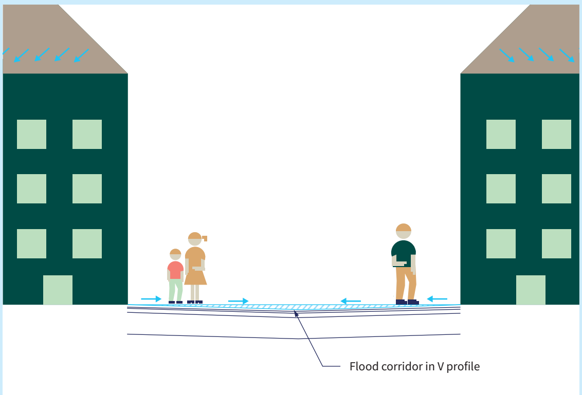
FIGURE 6-8 Example of a pedestrian street with V profile and no green structure.
